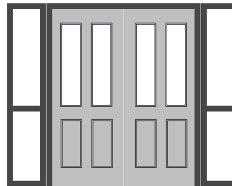
Double Doors with Glazed Sidelights and Midrails
